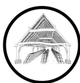
5. Drying the Bricks
